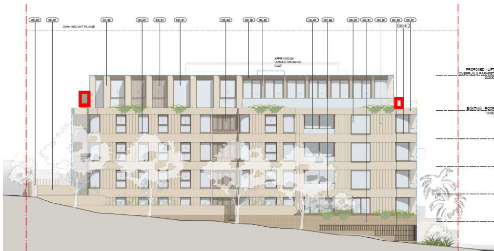
Figure 26: Proposed Side (East) Elevation - balcony extension (right) and air conditioning units (left) located outside building envelope of existing consent highlighted in bold red
