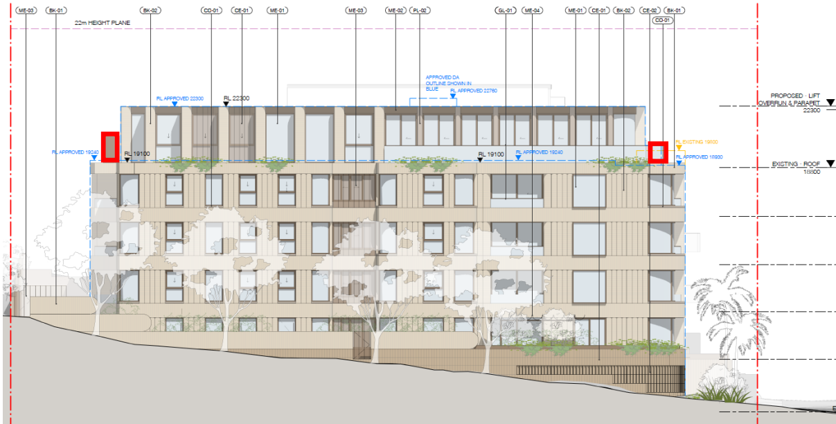
Figure 19: Proposed Side (East) Elevation (balcony extension and air-conditioning units located outside building envelope of existing consent highlighted in solid bold red) - changes to Level 4 lower rooftop parapet level shown outside blue dotted line
